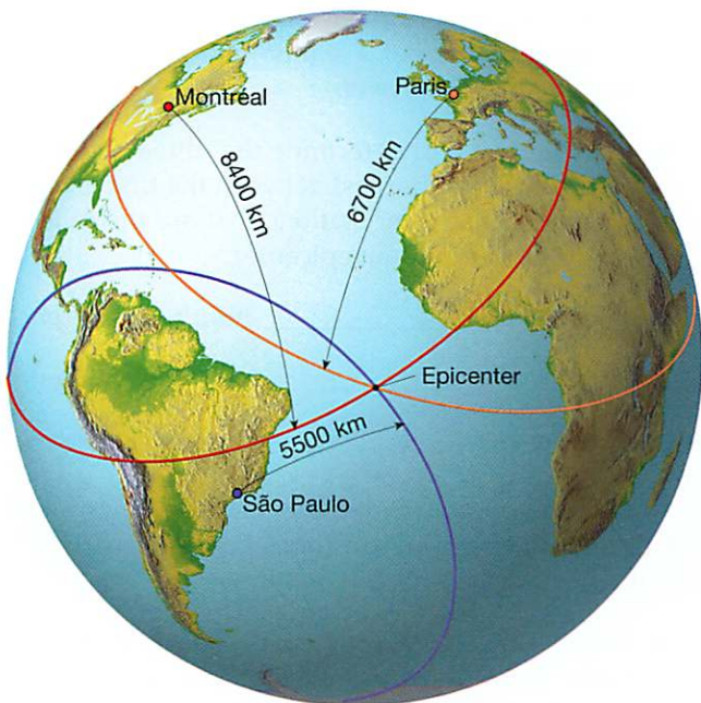
Figure 8.6 An earthquake epicenter is located using the distances obtained from three or more seismic stations.
