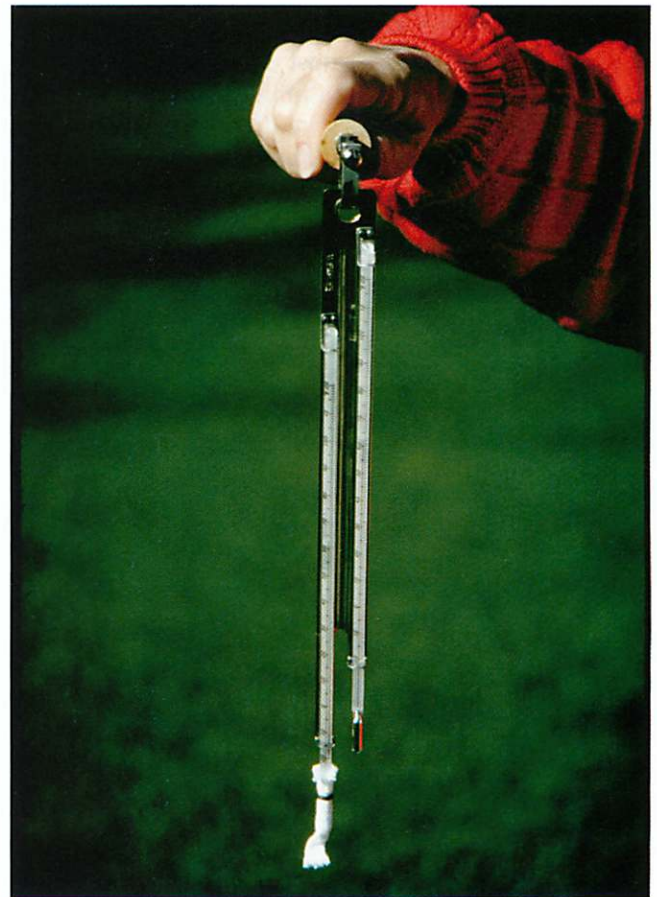
Figure 14.6 Sling psychrometer. The sling psychrometer is one instrument that is used to determine relative humidity and dew-point temperature. (Photo by E. J. Tarbuck)
