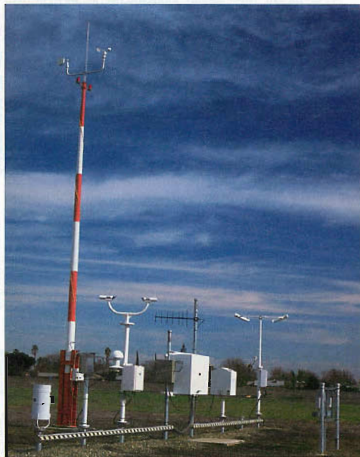
FIGURE 1.5 Gathering data and making careful observations is a basic part of scientific inquiry. A. This Automated Surface Observing System (ASOS) installation is one of nearly 900 in use for data gathering as part of the U.S. primary surface observing network. (Photo by Bobbe Christopherson) B. These scientists are working with a sediment core recovered from the ocean floor. Such cores often contain useful data about the geologic past and Earth’s climate history. (Photo by Science Source/Photo Researchers, Inc.)
