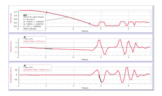
Observations: We realized that if the motion sensor got to close to the cart fan or the roller cart that it did not read correctly so we had to position it at a perfect distance in order to get a realistic graph.
