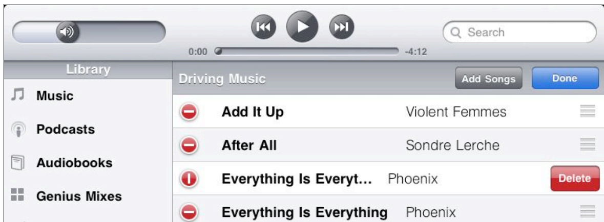
Figure 37: Deleting a track from a playlist requires two taps, to ensure you don't accidentally remove an item.
