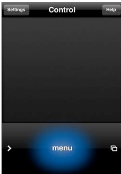
Figure 73: Welcome to the most boring figure in this book! What you don't see is that the entire empty field in the center of the screen acts as a trackpad. Here, I'm tapping (illuminated in blue) the Menu button.
