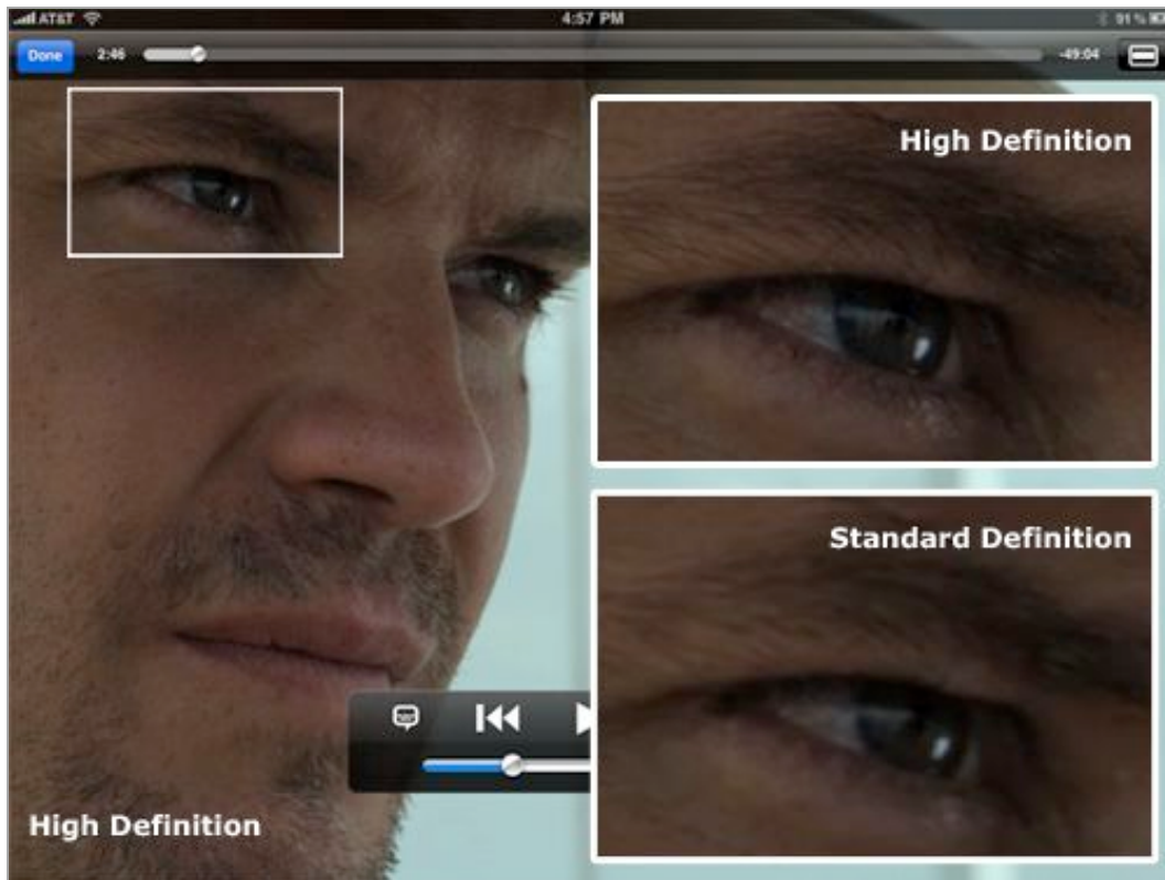
Figure 40: Compare iPad screenshots of a frame from the HD and SD versions of the same video; the detail boxes are shown at actual pixel size, taken from a screenshot. You can see sharper contrast in the hairs of the eyebrow in the HD version, while the SD version appears soft.
