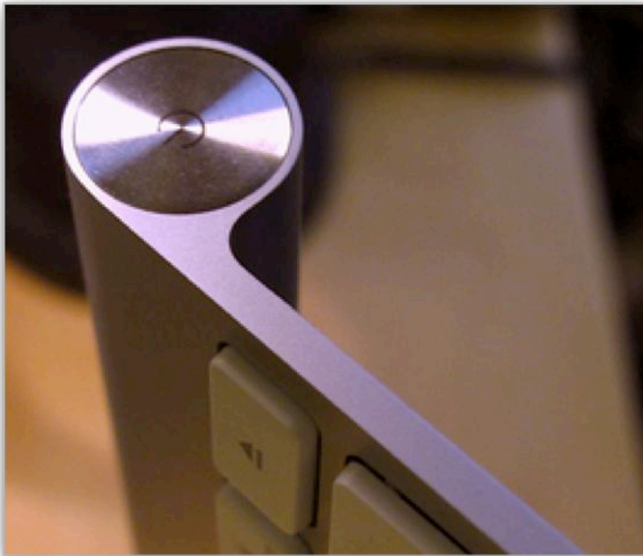
Figure 19: The power button is located on the right upper side of the Apple Wireless Keyboard.
