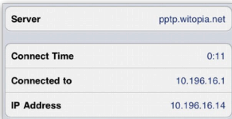
Figure 78: Connection details reveal a little more information about where the VPN terminates.
