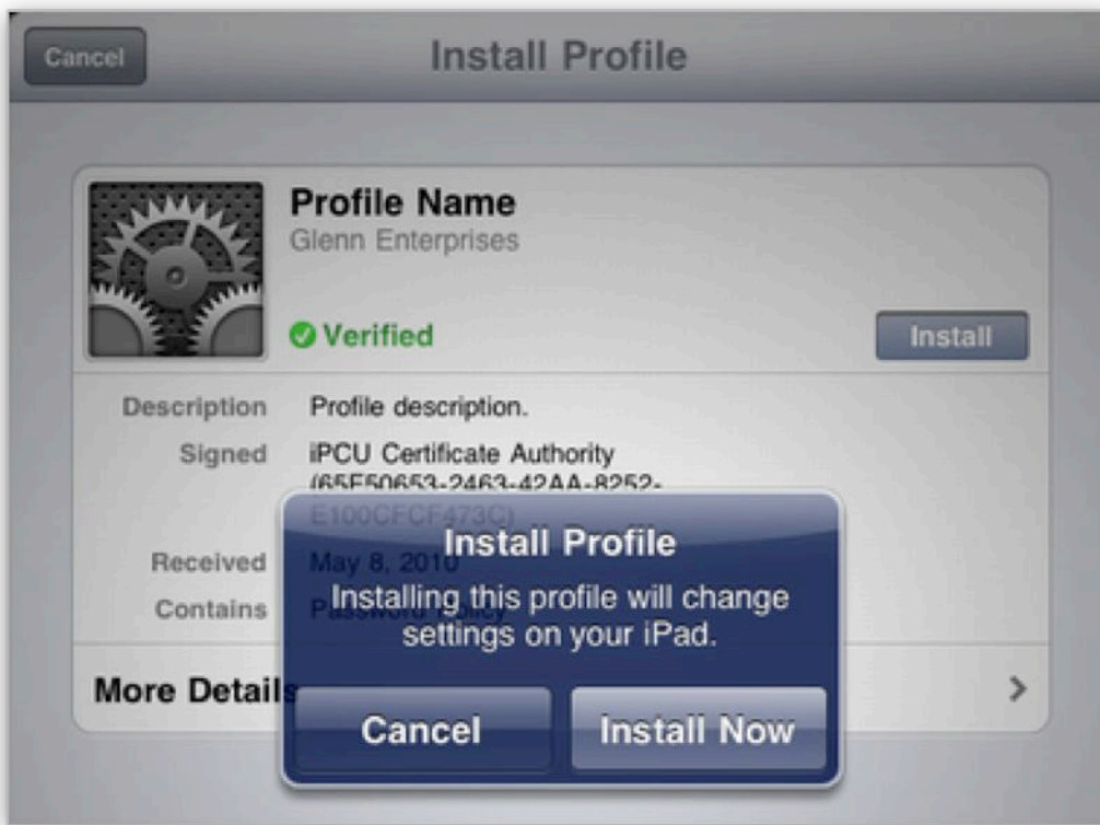
Figure 81: Tap Install Now to add the stronger passcode configuration you set in the utility.
