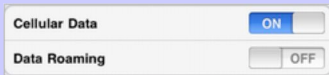
Figure 3: The Cellular Data switch lets you turn 3G service on or off separately from Wi-Fi networking. Data Roaming affects international use.
