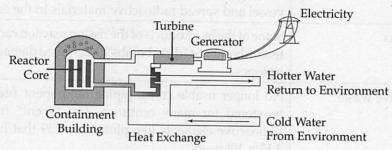
Pressurized Water Reactors—These reactors use the heat from the core to heat a
