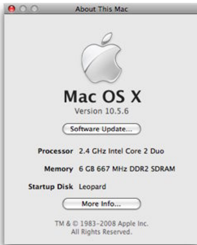
Figure 6: Choose  > About This Mac to display a window showing your Mac model, operating system version, and other details.
