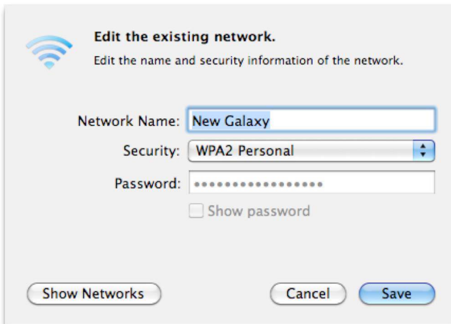
Figure 56: With the edit option, you can change the network name, security type, and password without re-selecting the network.
