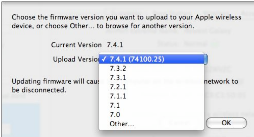
Figure 121: You can choose firmware that's stored in AirPort Utility, or choose a separate firmware file.
