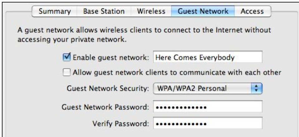
Figure 110: Guest Network view lets you set options for visitors to use your Internet connection without accessing your main network.
