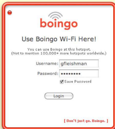
Figure 52: Boingo's software recognizes a network that's part of its plan and prompts a login.
