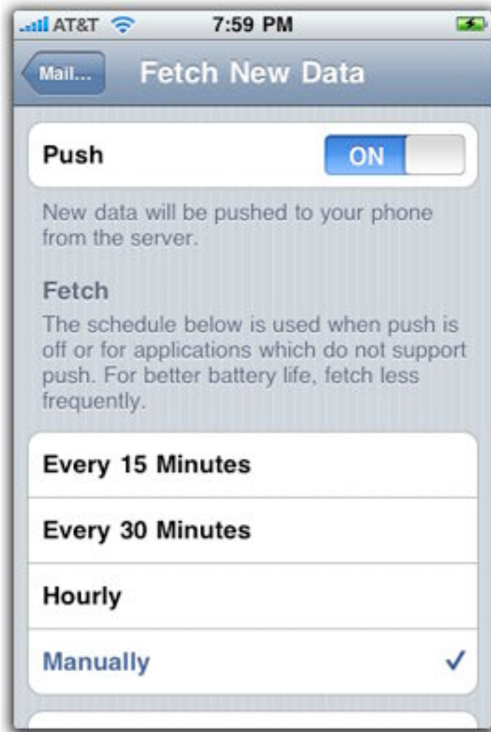
Figure 24: Data can be pushed from a service such as MobileMe or fetched from the device.
