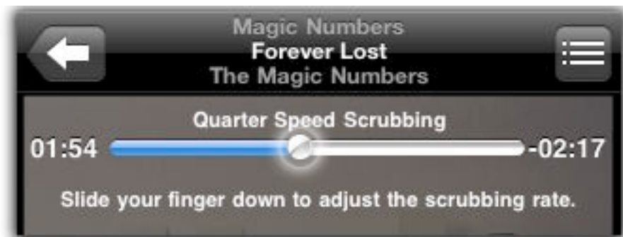
Figure 60: Scrub in fine increments by first sliding your finger down the screen, then dragging left or right.
