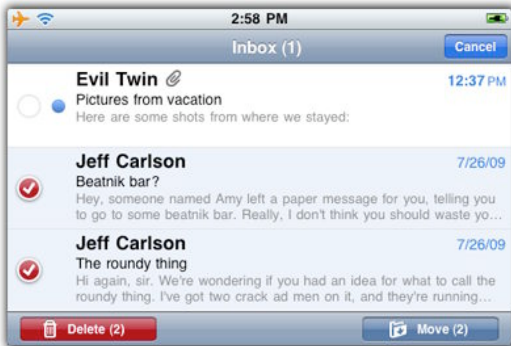
Figure 28: Select multiple messages and either delete them or move them to a new folder.
