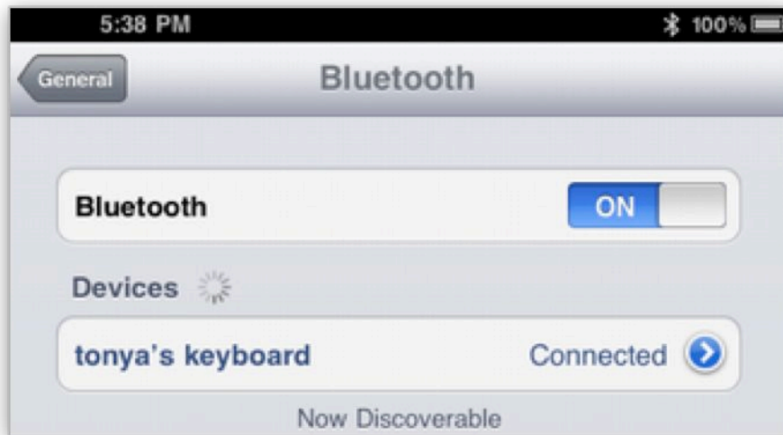
Figure 13: The keyboard appears in the Devices list with a “Connected” label, meaning that it is paired and in range. The Bluetooth icon in the status bar has turned white, indicating that Bluetooth is on and at least one device is connected.
