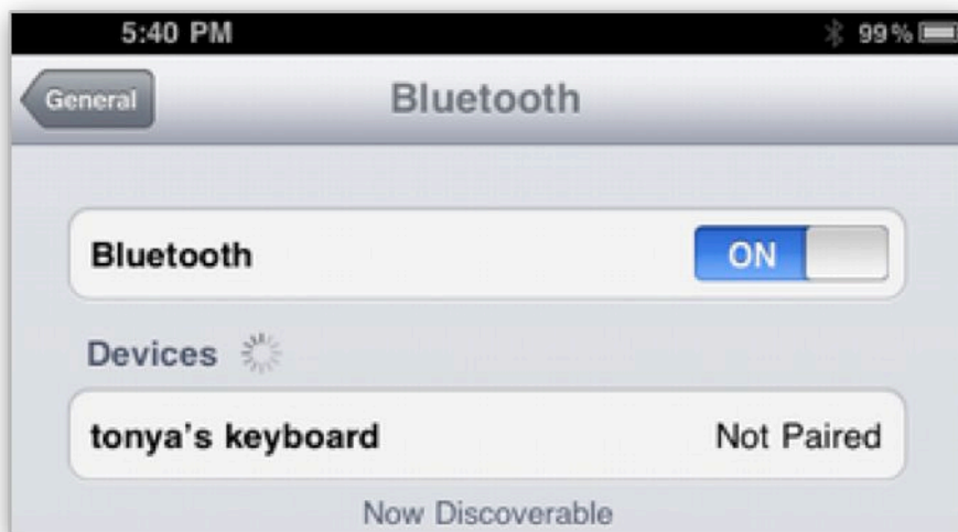
Figure 12: Discoverable devices appear in the Devices list. Notice the faint Bluetooth icon in the status bar by the battery indicator. The gray icon means that Bluetooth is on, but nothing is connected.
