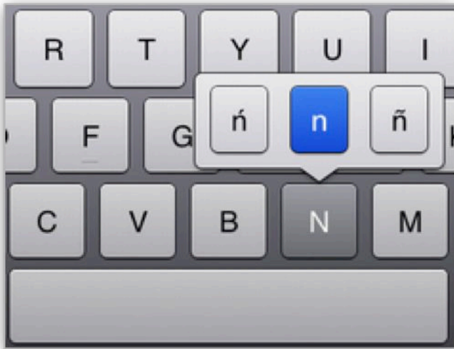
Figure 11: Touching and sliding combine into a fluid gesture for typing alternate characters.
