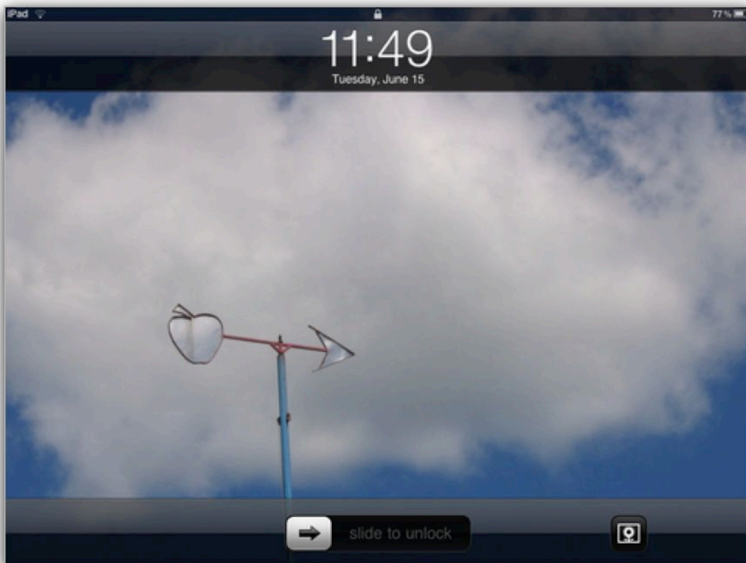
Figure 8: Here is my Lock screen, customized with a personal photo. Notice the "slide to unlock" slider (bottom, center) and the Picture Frame button (lower right).
