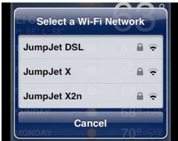
Figure 37: The Select a Wi-Fi Network list pops up when there are Wi-Fi networks in your vicinity but none to which you automatically connect.
