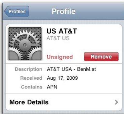
Figure 36: The details of an installed configuration profile.
