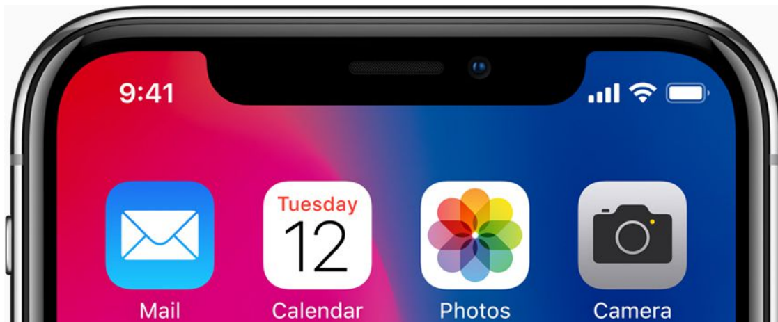
Figure 12: Other than the “notch” in the top-center, the iPhone X’s display spans the length and height of the device. Note the two “ears” on each side of the notch.
