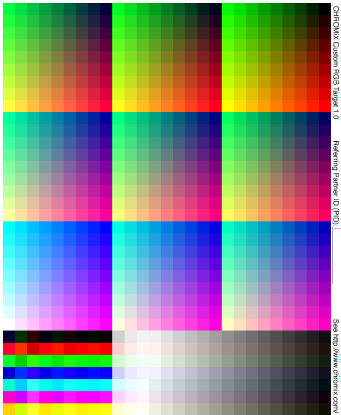
RGB Target file supplied by Chromix Color Valet, used to measure the printer, ink and paper performance together.
