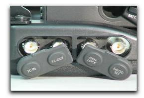
The Canon XL H1 (pictured above) has jacks for both timecode input and output which make it an ideal camera for multicam shoots.
