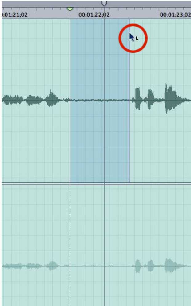
Figure 6. By moving the mouse to the top of the screen, a little "L" appears, indicating that we can make a selection on just the left channel of a linked pair.
