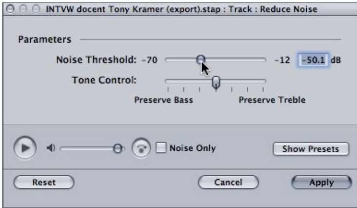
Figure 8. Noise reduction is a trade-off between reducing noise and affecting the remaining sound you want to keep.
